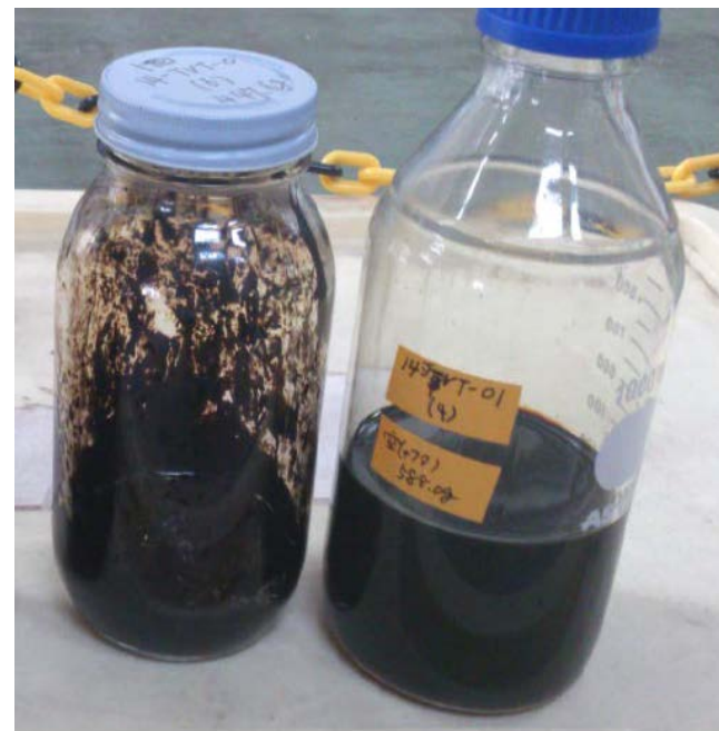
Products: Pitch (left side) and SCO (right side) (After 395 degC SCW Cracking)
