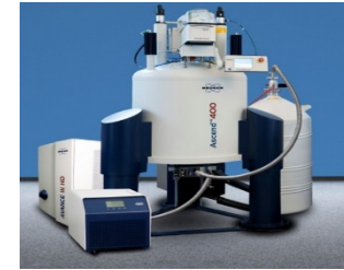
Nuclear magnetic resonance spectrometer of Bruker AVANCE III 400 MHz
